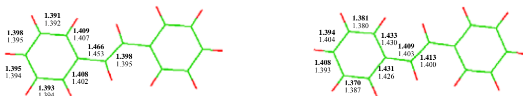
Fig 2. Optimized geometries for the ground (left) and lowest singlet excited state (right) of PPV2 ( 1 ). Upper values represent present calculation, lower ones from other computation (Reference 8).
