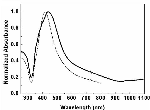
Figure 2. Absorption spectra of low density (dotted curve) and high density (solid curve) solutions of nanorods
