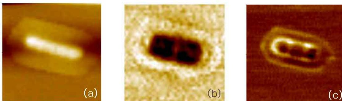
Figure 3. (a) The topography and (b, c) near-field scanning absorption images of a silver nanorod. Probe wavelength are 792 ~ 846 nm for (b) and 635 ~ 695 nm for (c), respectively. Image sizes:  $1.5\ \mu\text{m} \times 1.5\ \mu\text{m}$ .
