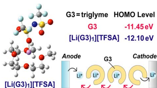
Fig. 2. The most probable structure of [Li(G3) 1 ][TFSA] ([TFSA] = [N(SO 2 CF 3 ) 2 ] - ) and the highest occupied molecular orbital (HOMO) energy level lowering of G3 in the probable structure, estimated by ab initio molecular orbital calculations, and schematic representation of ligand exchange conduction mode typically seen when electrochemical reactions occur at the electrode-electrolyte interfaces.
