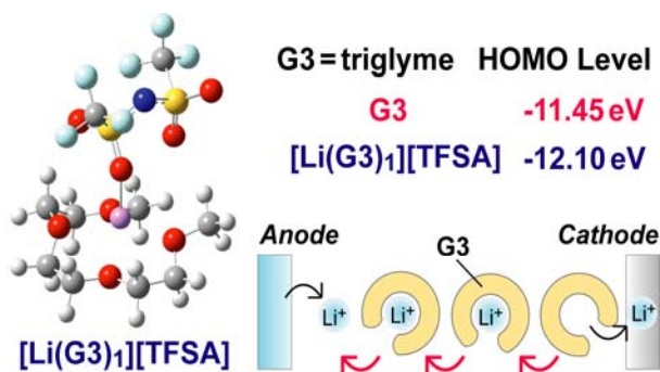
Fig. 2. The most probable structure of [Li(G3) 1 ][TFSA] ([TFSA] = [N(SO 2 CF 3 ) 2 ] - ) and the highest occupied molecular orbital (HOMO) energy level lowering of G3 in the probable structure, estimated by ab initio molecular orbital calculations, and schematic representation of ligand exchange conduction mode typically seen when electrochemical reactions occur at the electrode-electrolyte interfaces.
