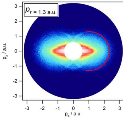
**Fig. 1.** An angle-resolved rescattering photoelectron spectrum of  $C_2H_6$ .
