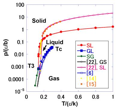
Phase diagram in the (p, T) space. The calculated result is compared with the experimental data on argon, the EOS and the free energy calculation. Tc and T3 are the critical point and the triple point.
