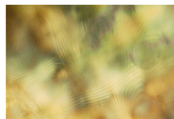
Fig.2 Photograph of cholesteric lyotropic liquid crystalline phase of PTPALG in TCE at 120°C
