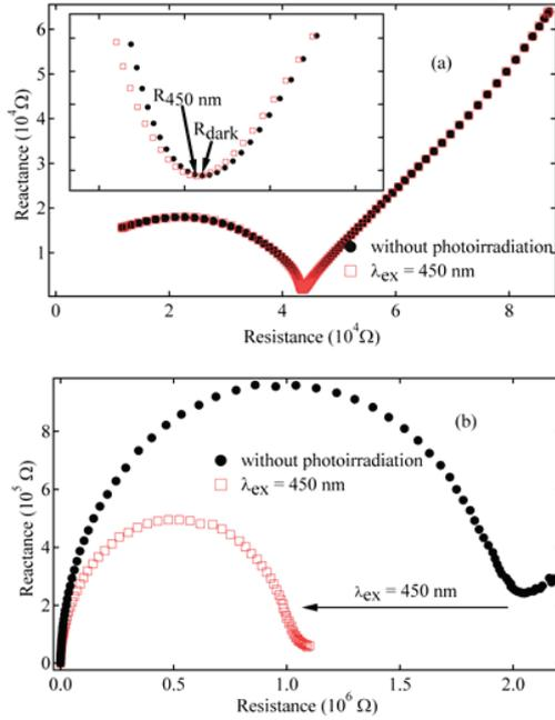
Fig 2: Cole-Cole plots of polycrystalline  $\gamma$ -AgI (a) and  $\beta$ -AgI (b) with ( $\square$ ) and without ( $\bullet$ ) photoirradiation at 450 nm measured by the ac method. The inset of (a) is the expansion of Cole-Cole plots in the bulk resistance region indicating the shift of the Cole-Cole plots with photoirradiation.
