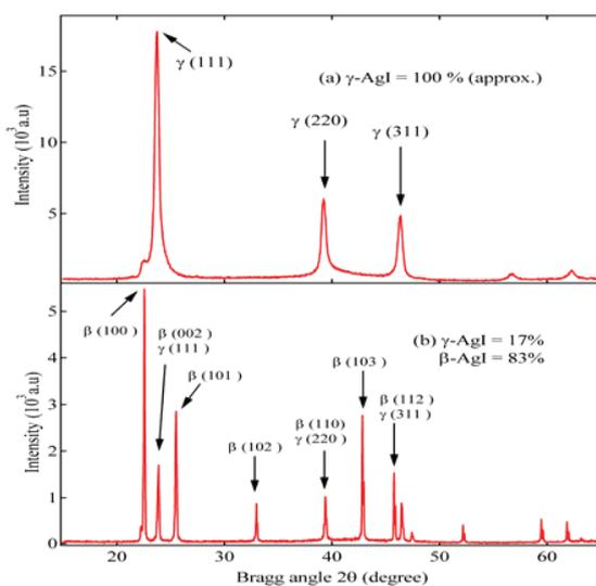
Fig 1: XRD pattern of  $\gamma$ -AgI (a) and  $\beta$ -AgI (b).
