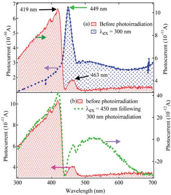
Fig 3: Photocurrent excitation spectrum of polycrystalline  $\gamma$ -AgI following the photoirradiation at 300 nm and at 450 nm indicating the red and blue shifts of the exciton band, respectively.
