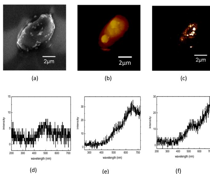
Figure 1. (a) SEM image of a dried yeast cell conjugated to triangular gold nanoplates. The mean base-length of the triangles is about 300nm. (b) Topographic image of the same cell taken by the SNOM apparatus. (c) Near-field two-photon excitation image of the same cell. Excitation: 780 nm. (d) to (f) Typical spectra of TPIPL from the sample. The spectral region longer than 710 nm was cut off by the filter.
