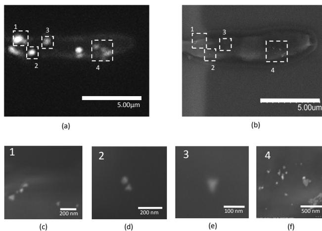
Figure 2. (a) TPIPL image of cells conjugated to triangular gold nanoplates taken by a TPLSM. Incident laser power was 1 mW. The base lengths of the plates were mostly in the range between 70 and 100 nm. (b) SEM image of the same cells. (c) to (f) Enlarged SEM images for the luminescence spots marked in (a) and (b).
