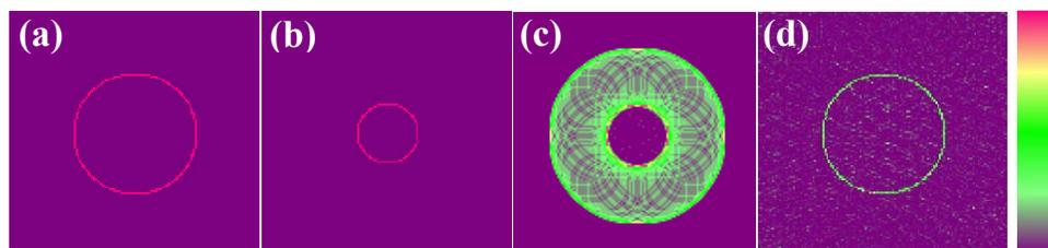
**Fig.-2:** (a)–(b) 2D original images (circles with radii 31 and 15 pixels, respectively); (c) Noise-mixed convolved image with blurred width of 30 pixels and (d) Recovered Image (same as (a) except noise blurred); Image size:  $128 \times 128$  pixels.
