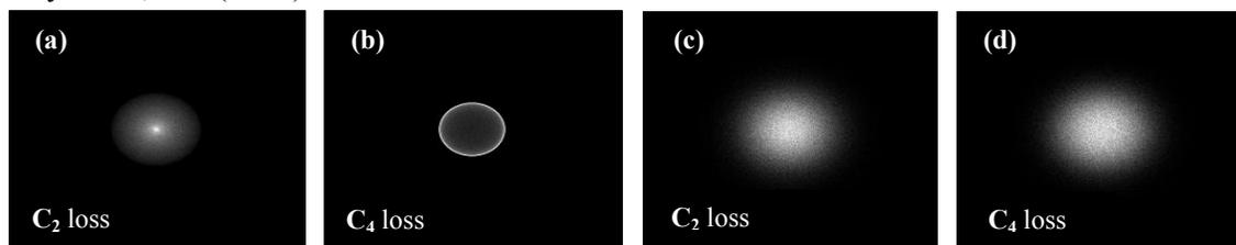
**Fig. 1:** Simulated 2D projections of the 3D scattering distributions of  $C_{56}^+$  fragments (image size:  $40 \times 40$  mm). (a) and (c), sequential ejection of  $C_2$  units; (b) and (d), Fission of  $C_{60}^+$ . The beam temperature is 0 K for (a) and (b) and 273 K for (c) and (d).
